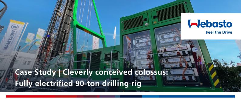
Dutch manufacturer Dieseko, in collaboration with Webasto and partner Danfoss Editron, venture into electrification of a giant Woltman drilling rig. The civil engineering machine weighs in at 90 tons and can drive piles of up to 36 meters in length into the ground by drilling or driving.
