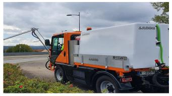
"The batteries are manufactured in Germany and give LADOG the flexibility required for use in this class of vehicle." The two standard battery systems installed fulfill two cornerstones of the requirement profile: losing as little cargo space as possible while maintaining a low center of gravity for driving over a curb. "This ensures the safety and stability of the vehicles," says Freudenreich.
